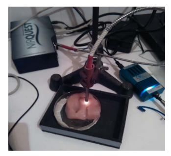
Figure 1. Measuremet of meat samples using a reflection fiber-optic probe and portable scanning NIRQuest 512 instrument
