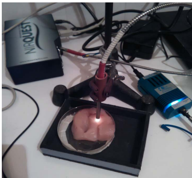
Figure 1. Measurement of meat samples using a reflection fiber-optic probe and portable scanning NIRQuest 512 instrument
